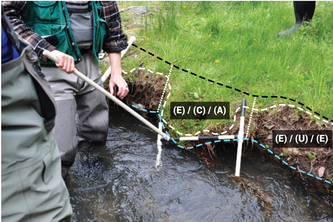
Figure H.12. The stability and cover plot extends vertically up the bank from the scour line (blue dashed line) to the edge of the first bench (dark dashed line). The frame rests on erosional, covered (E/C) bank (white dashed line, greenline). Immediately right and left of the frame, the bank is erosional (E) and uncovered (U). The vertical, uncovered streambanks would be evaluated as eroding (E) and covered bank as absent (A).
