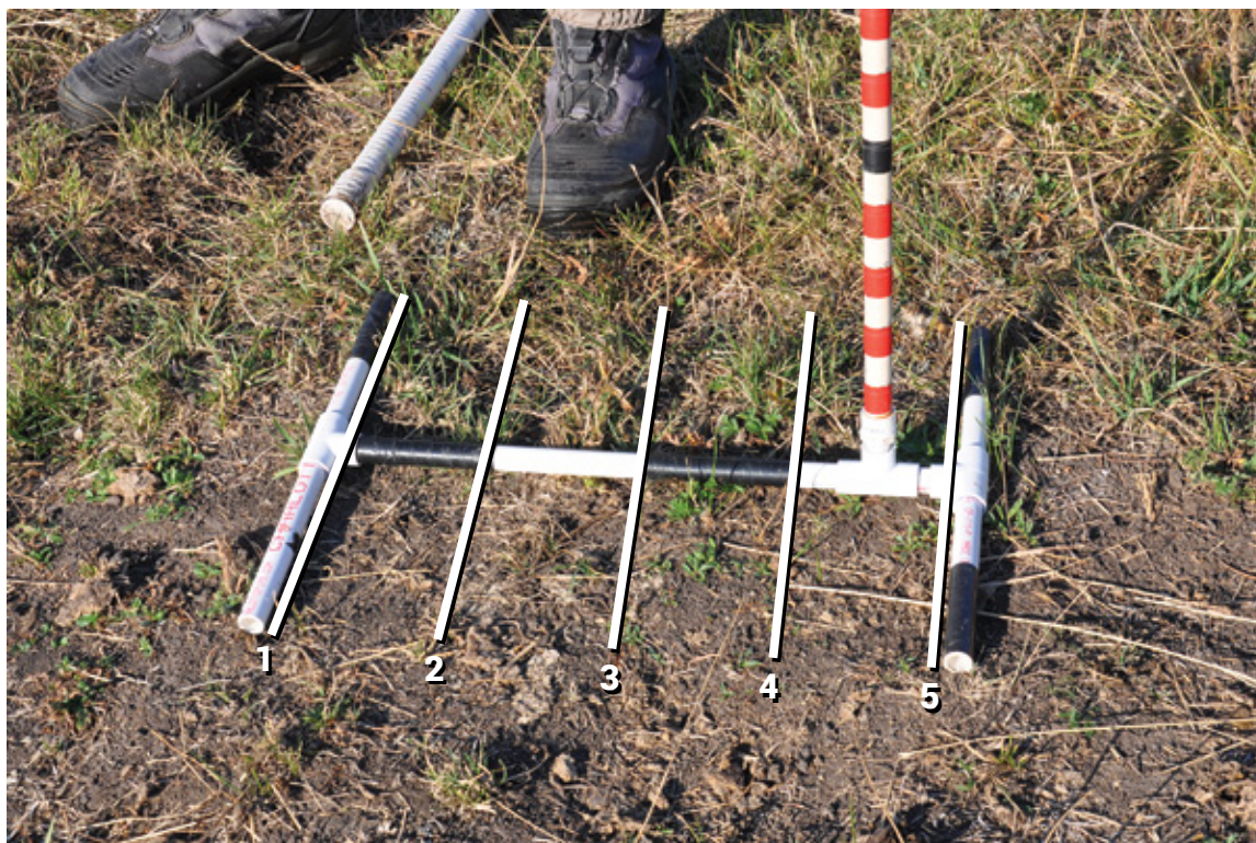
Figure E.5. This frame falls along a compacted and unvegetated trail. Although there are no depressions greater than 13 mm, the compacted trail intersects all 5 observation lines on the near half of the frame, so 5 alterations would be recorded.
