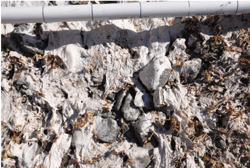
Figure 71. Measuring substrate when dried algae cover the substrate. Dried algae may form a mat covering the substrate. Although obvious when the channel is dry, inundated algae can be mistaken for fine sediment; measure inorganic substrate only.
