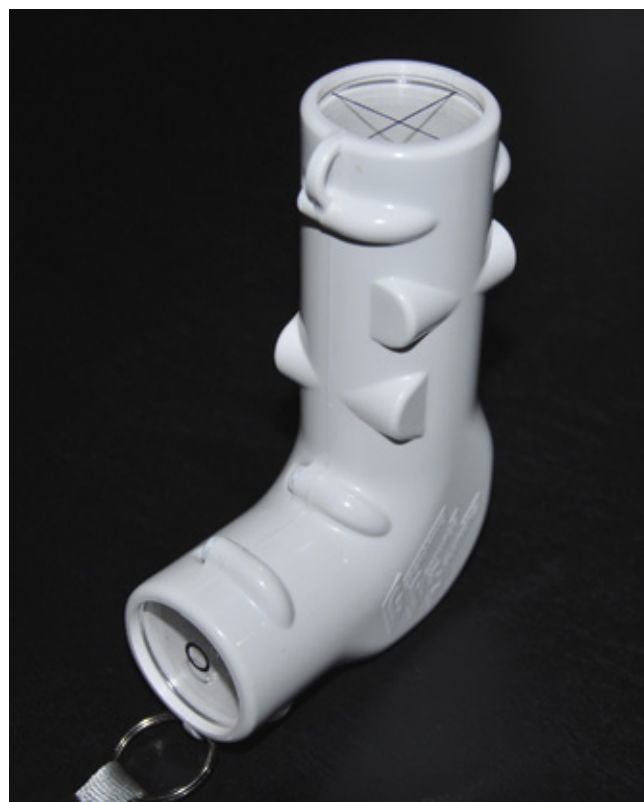
Figure 20. A densitometer. Densitometers provide a bull's-eye leveling bubble and sighting cross hairs to determine if overstory plants are directly overlying sampling quadrats.
