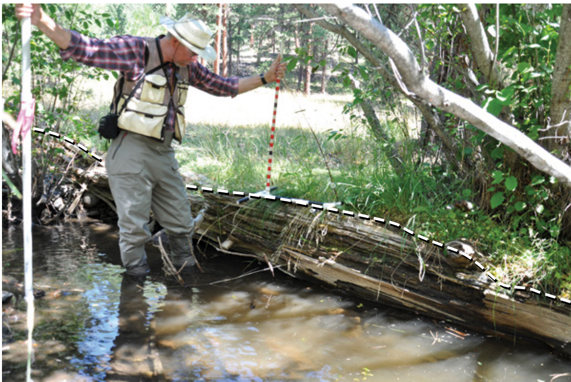
Figure D.11. Anchored wood includes dead woody material that is not likely to move during high flows, has no evidence of erosion behind it, and is above the scour line. Here, the greenline follows the top edge of the anchored log.
