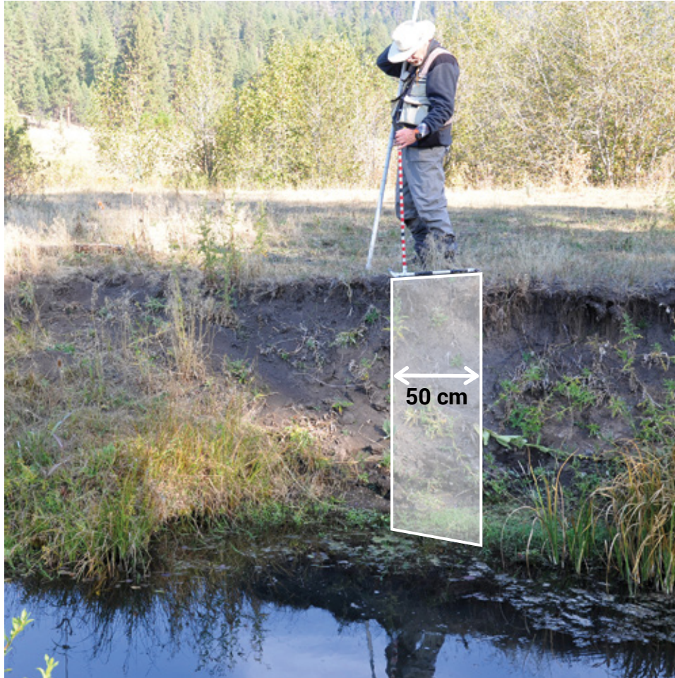
Figure 55. Positioning the streambank stability and cover quadrat from the scour line to the lip of the first bench. The quadrat to evaluate streambank stability and cover extends from the scour line (or water's edge or edge of the active channel) to the lip of the first bench. The quadrat is oriented straight up the bank and is 50 cm long (i.e., the length of the MIM frame).
