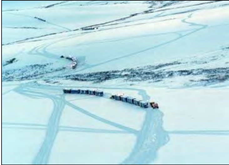
Figure 3g.7. Strings of sled-mounted trailers (Cat trains) being moved during 3-D seismic exploration in foothills terrain near Kavik, west of the Arctic NWR, 2001. The Cat trains in the background apparently required two tractors per train to travel in this hilly terrain (one D7 to assist the lighter tractor), while the two trains in the foreground were waiting for tractors to return for them. Photo courtesy U.S. Fish & Wildlife Service.
