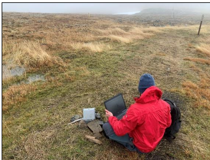
Figure 3: Downloading data from a soil temperature monitoring station used to assess the impacts to permafrost soils from off-highway vehicle use.
