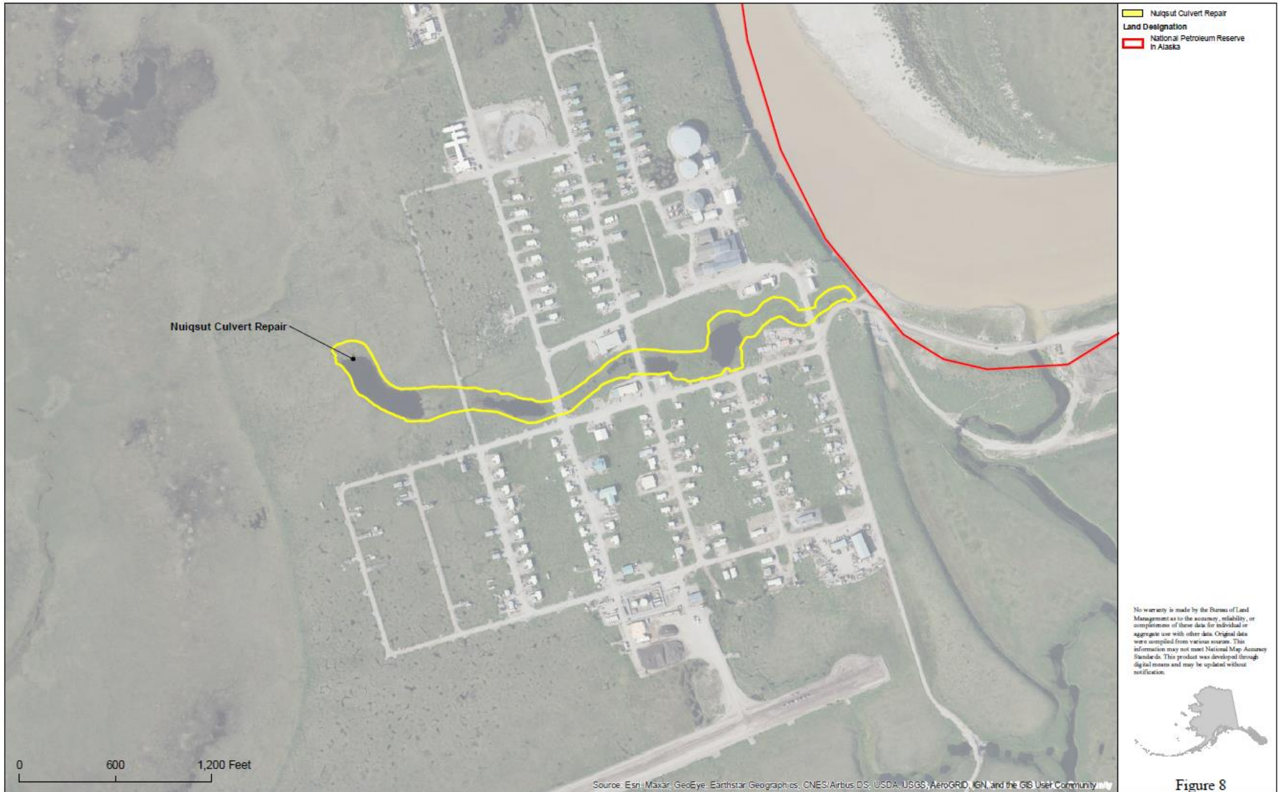
Figure 2.4. Proposed voluntary culvert repair to enhance 11.8 acres (0.05 km 2 ) of Waters of the U.S. abutting the Nigliq Channel of the Colville River near Nuiqsut, Alaska.
