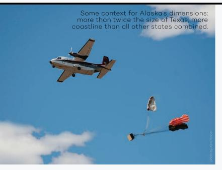
Once the cargo is out the rear door, the pallet is falling 8 to 12 feet per second with the aid of the massive round parachutes—three or four depending on the weight.
