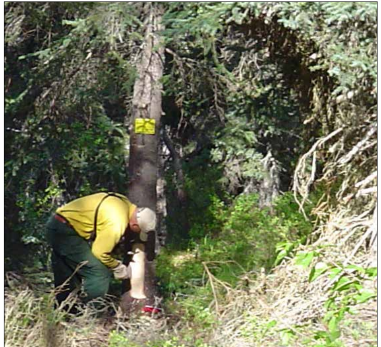
Surveyor scribing a bearing tree in southeast Alaska.
