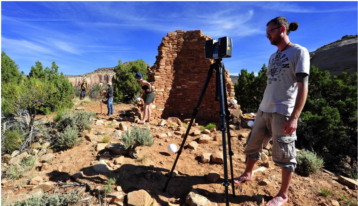
Archaeological students from Jagiellonian University digitally mapping and LiDAR scanning at the “Mad Dog Tower” (5MT135), CANM, Colorado.
