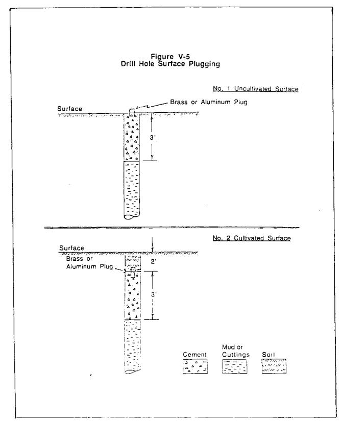
Accordingly, upon completion of each drill hole, the operator will (1) properly plug and abandon the hole, or (2) condition the hole for use as a water well, or (3) condition the hole for retention as a monitoring well.
