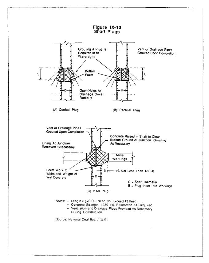
Plugs may incorporate pipes through which water from the upper part of the shaft can be drained into the workings below during construction. The drain pipe is grouted off after the drain pipe has had a chance to cure and after formation and contact grouting has been completed. Ventilation is an important consideration.
