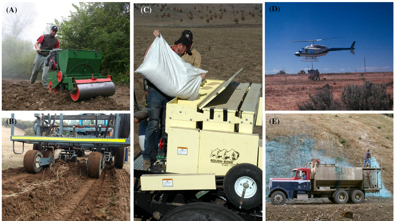
Figure 4 Seeding equipment: (A) Motorized seed mix delivery broadcaster for small-scale projects. This broadcaster provides some degree of seed-to-soil contact but requires a prepared seed bed (Romagnese, Italy). (B) Custom-made precision seeder for delivery of seed mixes used in reconstruction of farmland to the local reference community in southwestern Australia. (C) Minimum-till drills reduce surface disturbance. The triple seed box provides for separate seeding and even flow of large, small, and fluffy seeds. (D) Helicopters can seed irregular areas in rugged terrain and do not require a landing strip. Seed in the rotary spreader is dropped onto a spinner for distribution, but spread is affected by flight elevation, wind, and seed characteristics. (E) Hydroseeding a road cut in Oregon, U.S.A. Photos: (A) S. Pedrini, (C, E) U.S. Forest Service, (D) H. Wiedemann.
